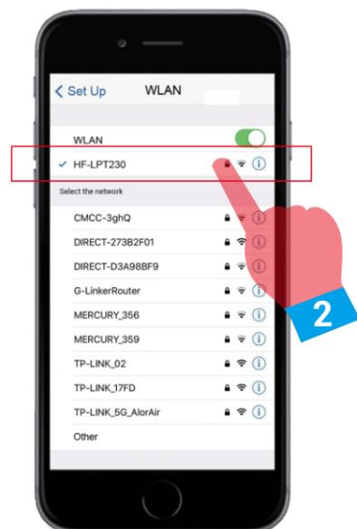
**2** For new users, if there is no network, they can choose direct connection mode. (Make sure you are connected to the HF-LPT230 hot spot) then click the Connect button. Then click I have connected successfully.
