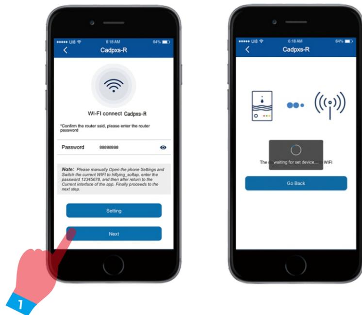
**9** After the WI-FI connection is successful, the name of the connected dehumidifier will be displayed on the interface, and then click the next step to enter the home page. The main interface will automatically connect to the FOFE6BEF6D7C dehumidifier.
