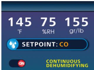
The display will communicate to the user that the machine is continuously dehumidifying on the last line of the dashboard.
